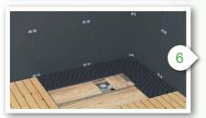
Spread the adhesive evenly over the area where the shower tray is to be installed, being careful to clean away any adhesive on the rim of the trap.
