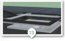
Use the riser piece to balance the height difference between tile and drain.
