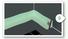
Seal all joints (both wall and floor) utilising special waterproof membrane / paste.
